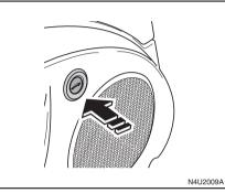
Press the remote trunk release button, located on the side of the driver's door trim, to release the trunk lid.
